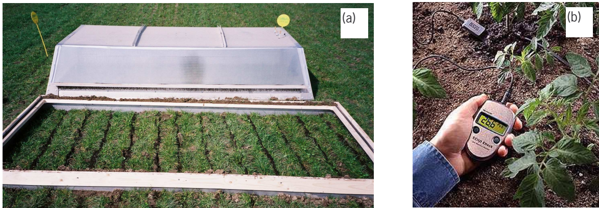
Figure 13 Measurement methods. (a) ECH 2 O Dielectric Aquameter Sensor (volumetric water content); (b) Flux chamber and permanent installed wooden frames (CH 4 and N 2 O fluxes)
